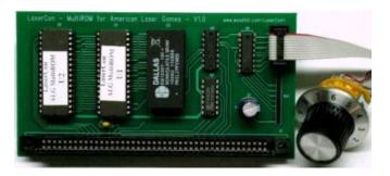
The LaserCon - ALG MultiROM board is a direct replacement for the original RAM/ROM board found on the light-gun arcade machines produced by American Laser Games (Arcade version only, based on the Amiga 500 computer, manufactured from 1990 through 1994).
